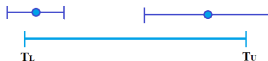
Fig. 1. The measured values, accompanied by measurement uncertainties, whose values exceed the tolerance interval's limits.
